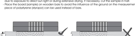
**6.2 Veneer MC measurement procedure**
